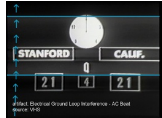
Electrical Ground Loop Interference:
