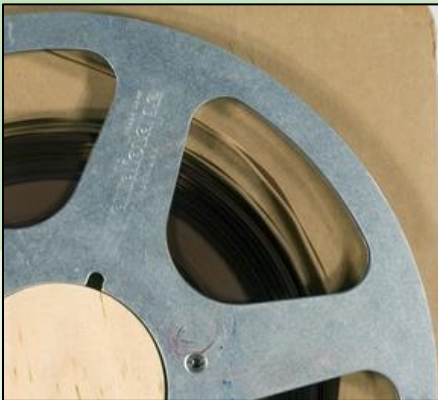
Tape is deformed.
