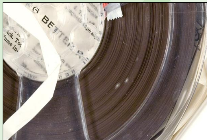
Open reel tape with mold or mildew.
