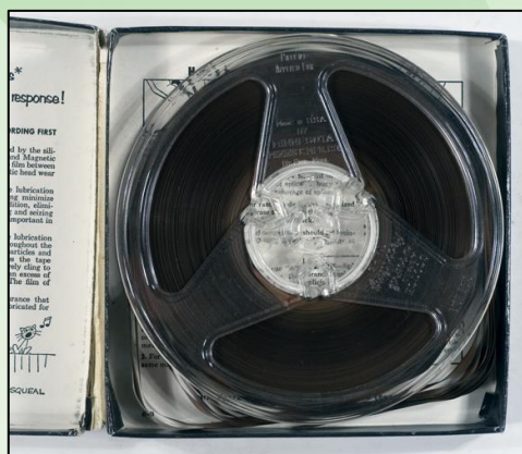
No sign of mold or oxide flaking.
