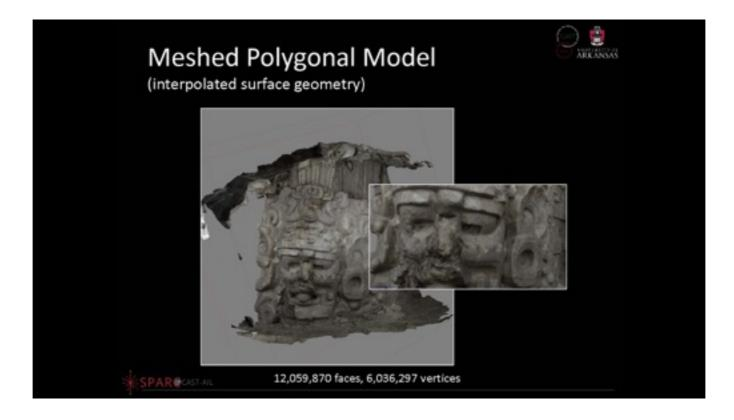
Next, the software will generate a triangular mesh by joining the points together. In this model, there are now over 12 million faces connected by over 6 million vertices. the final processing step is to add in the texture data, and will cover that result in another tutorial as well
