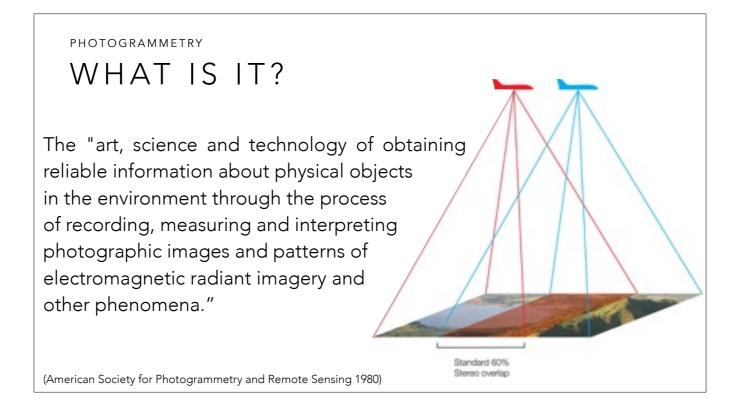
so what is photogrammetry? It's the...art, science and technology of obtaining reliable information about physical objects in the environment through the process of recording, measuring and interpreting photographic images and patterns of electromagnetic radiant imagery and other phenomena.
