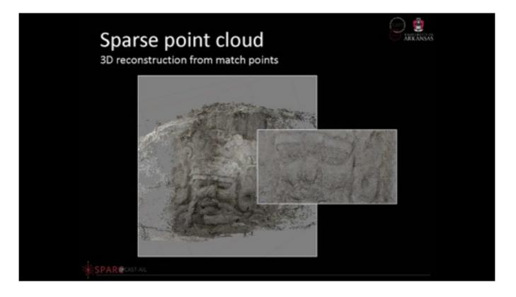
The next step is to generate the sparse point cloud. Believe it or not, this is as easy as clicking a button inside of the software. What you are seeing is not a photograph, but actually the underlying 3D data as a cloud of points
