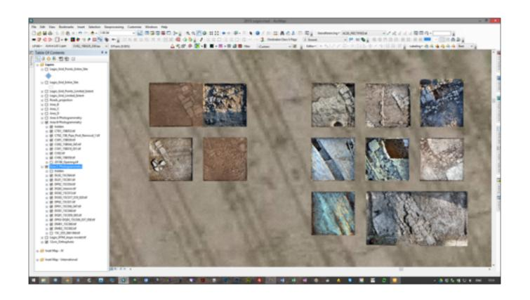
Generating two-dimensional, but precisely measured orthographic photographs is very useful for a variety of purposes, including GIS, or geographical information systems. Here, we have placed the ortho photos generated from our photogrammetry technique directly into our GIS. Because these 3D photographs have real world coordinate information inside of them, they slip right into the GIS perfectly. In other words, each of these images is perfectly aligned in real-world space.
